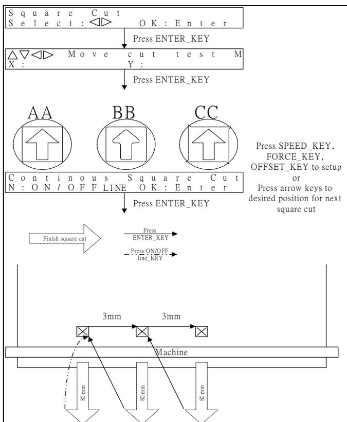
If the pattern appears to be BB or CC layout, press [OFFSET KEY] to adjust the offset value until AA pattern discovered.
