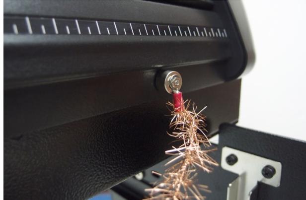
**Step 3** The Installation of conductive copper wires is done.
