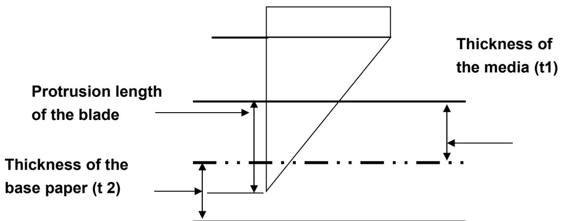
Length of protrusion =  $t_1 + t_2 / 2$ , but for your convenience you may just make it about 0.3mm ~ 0.5mm beyond the blade holder tip.
